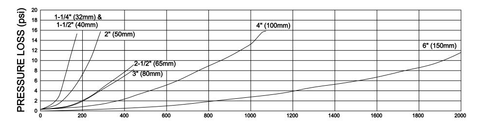
FLOW RATE (gpm)
