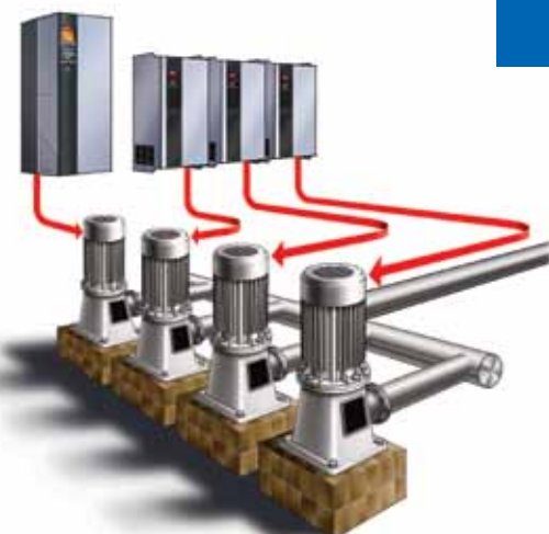
This illustration depicts a typical VLT® AQUA Drive installation utilizing the Cascade Controller option. The controller is being used in conjunction with MCD Series Soft Starters to operate one to four pumps as demand requires.
